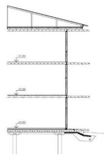
Figure 11: Original balcony construction, Alingsås
